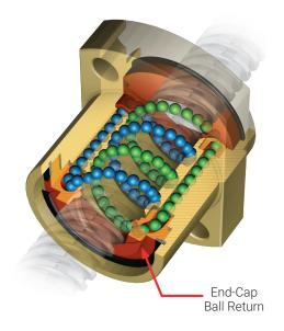
**End-cap return nuts** route the flow of ball bearings from one end of the nut to the other. This design provides increased speed options because of its ability to accommodate longer leads, which is not practical in the multiliner nut design.
