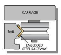
extrusions natural inaccuracies of bow, warp, twist and cambor. Hardened steel inserts are embedded into the specially designed extrusion for smooth, repeatable travel of the IVT carriage. The end result is the next generation of linear guide systems, IVT significantly reduces mounting components, fasteners and alignment installation time while ensuring precise linear motion travel at a lower total installed cost.
