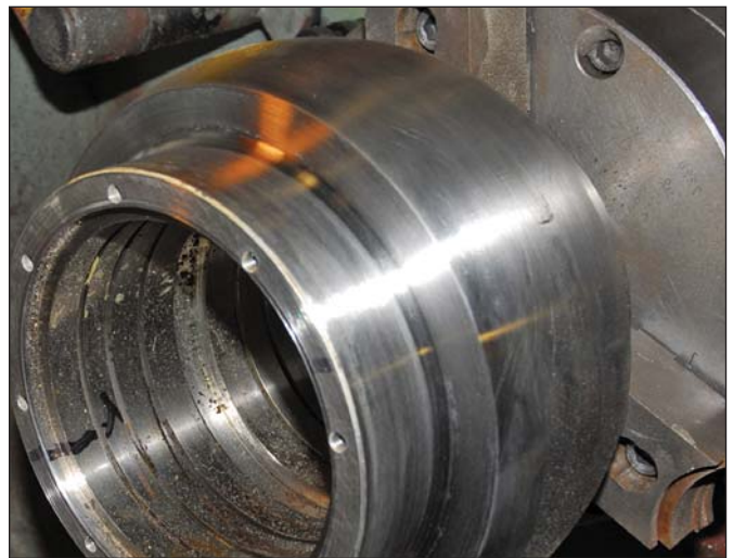
PBC Linear Doctor Bearing after 16 years of performance.
