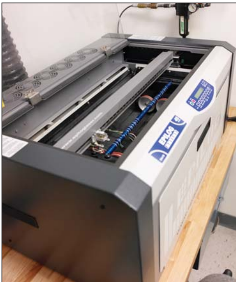
PBC Linear's solution provided subtle and precise adjustments at system's target mirrors.
