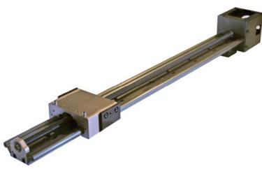
Manufactured by PBC Linear in Roscoe, Illinois, the Uni-Guide can be shipped as soon as the product is assembled. The Uni-Guide is carefully matched, carriage to rail, and hard aluminum anodized to support a long life-span. Also, with PBC Linear's patented self-lubricating technology, the Uni-Guide can provide contaminant free linear motion that never requires additional lubrication. This allows for a huge life-span cost savings for the customer.
